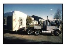
Modular homes are built to the state/local building codes of the jurisdiction where the home is going to be sited. These are the very same building codes to which site builders adhere. Modular homes are constructed of the exact same materials found in site-built residential construction.
