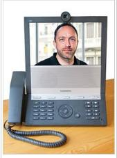
The Tandberg E20 is an example of a SIP-only device. Such devices need to route calls through a Video Communication Server to be able to reach H.323 systems, a process known as "interworking" (2009).
