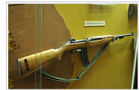
M2 Carbine, note: the selector lever on the left side, opposite of the bolt handle.
