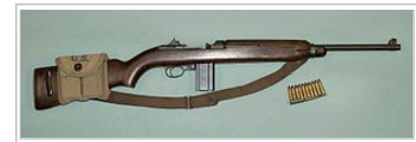
WW II M1 Carbine with a magazine pouch mounted on the stock that held two spare 15-round magazines
