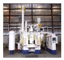
Ring & Pinion Gear Shot Peening Machines
