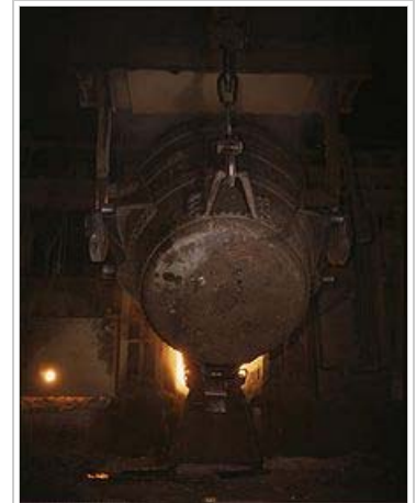
A ladle of molten iron is poured into an open hearth furnace for conversion into steel at Allegheny Ludlum Steel Corp., 1941
