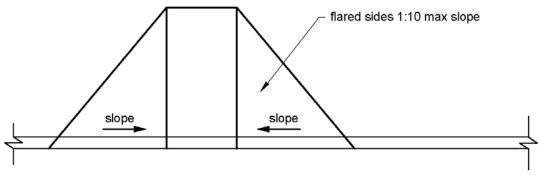
Figure 406.3 Sides of Curb Ramps
