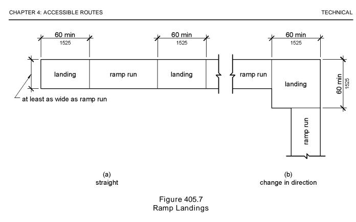
405.7.1 Slope. Landings shall comply with 302. Changes in level are not permitted. EXCEPTION: Slopes not steeper than 1:48 shall be permitted.
