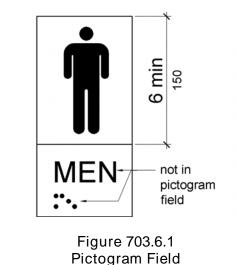
703.6.2 Finish and Contrast. Pictograms and their field shall have a non-glare finish. Pictograms shall contrast with their field with either a light pictogram on a dark field or a dark pictogram on a light field.
