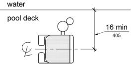
Figure 1009.2.2 Pool Lift Seat Location
