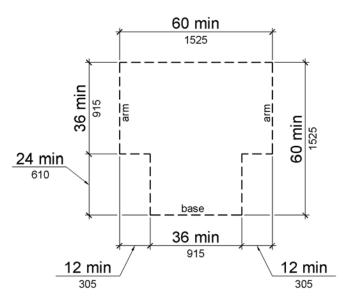
Figure 304.3.2 T-Shaped Turning Space
