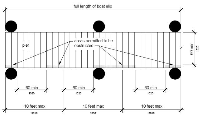
Figure 1003.3.1 Boat Slip Clearance
