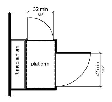
Figure 410.6 Platform Lift Doors and Gates
