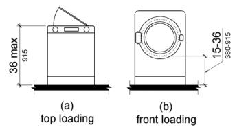
Figure 611.4 Height of Laundry Compartment Opening
