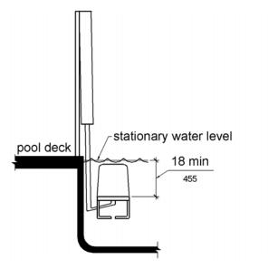
Figure 1009.2.8 Pool Lift Submerged Depth
