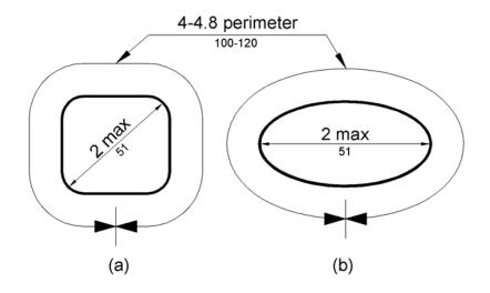
Figure 609.2.2 Grab Bar Non-Circular Cross Section
