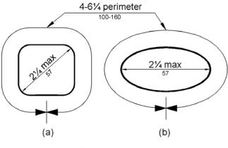
Figure 505.7.2 Handrail Non-Circular Cross Section
