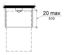
Figure 704.2.1.2 Forward Approach to Telephone
