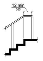
Figure 505.10.2 Top Handrail Extension at Stairs
