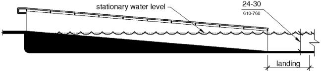
Figure 1009.3.2 Sloped Entry Submerged Depth
