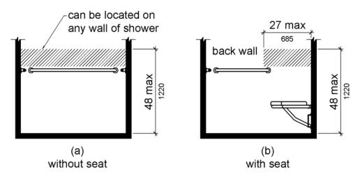
Figure 608.5.2 Standard Roll-In Type Shower Compartment Control Location
