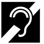
Figure 703.7.2.4 International Symbol of Access for Hearing Loss
