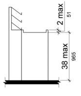
Figure 904.3.2 Check-Out Aisle Counters
