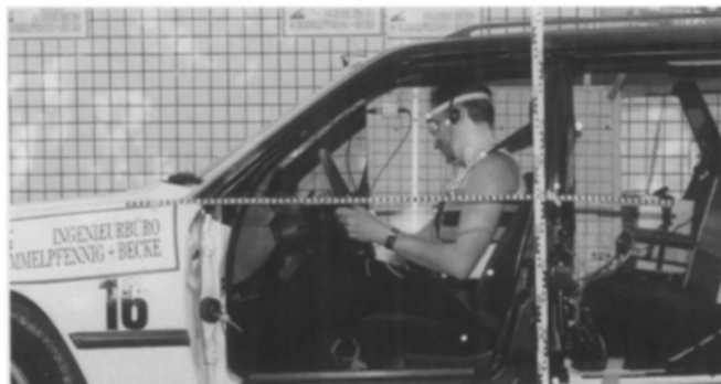
Fig. 2 Initial position of a male test subject immediately before a two-car collision. Note the blinds, the headset, and the leads connecting the test subject to biomechanical acceleration and electromyography (EMG) sensors
